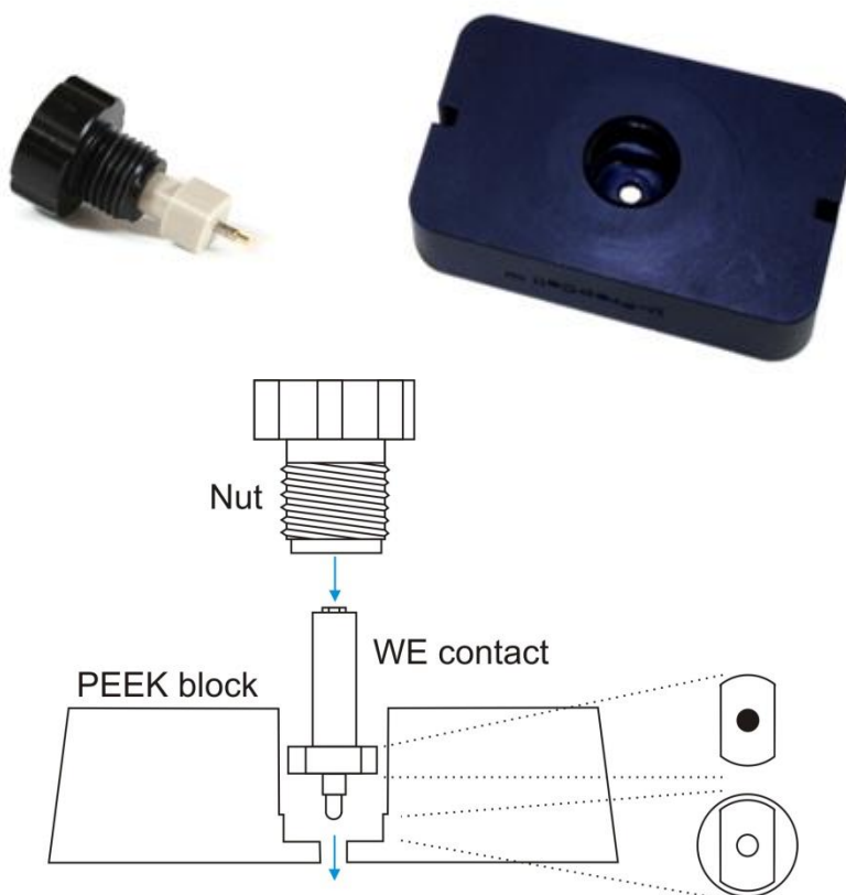
Figure 15. \mu -PrepCell – electrode contact, nut and electrode block. Below: schematic intersection
