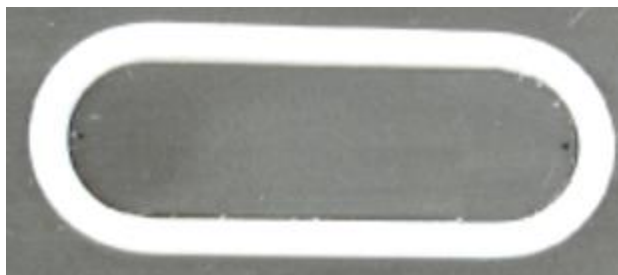
Figure 21. Active area of the \mu -PrepCell SS inlet block with Teflon O-ring.
