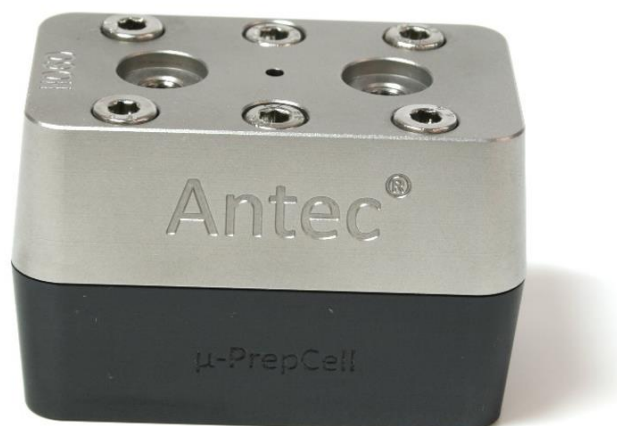
Figure 13. \mu -PrepCell inlet and WE block fixed with 6x M4 stainless steel allen screws.
